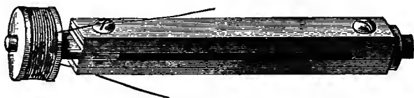
FIG. 47.—Single-pole compound bar telephone magnet.
